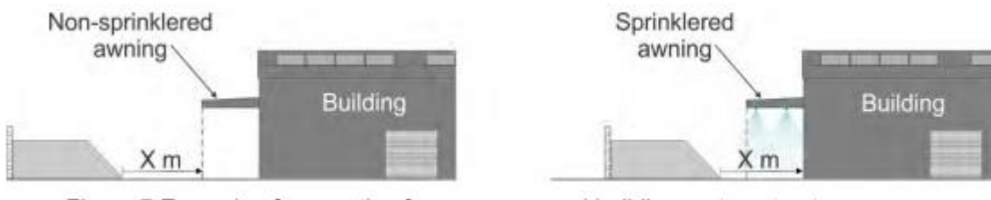
Figure 6 Example of separation between covered building part of structure
