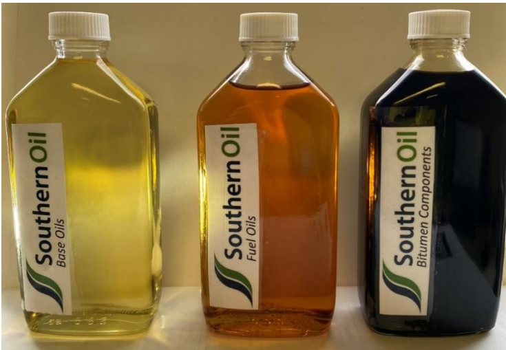
Multiple products recovered through the fractional distillation process. Image courtesy of Northern Oil.
